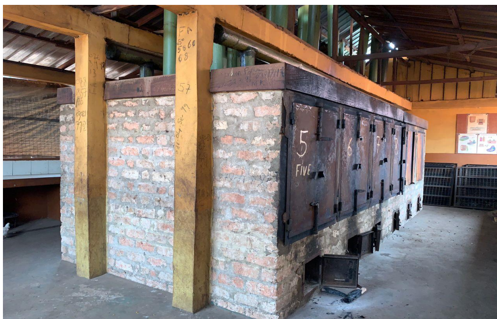
Figure 12: The Matis ovens as part of a system (consisting of 12 ovens at Tombo)
