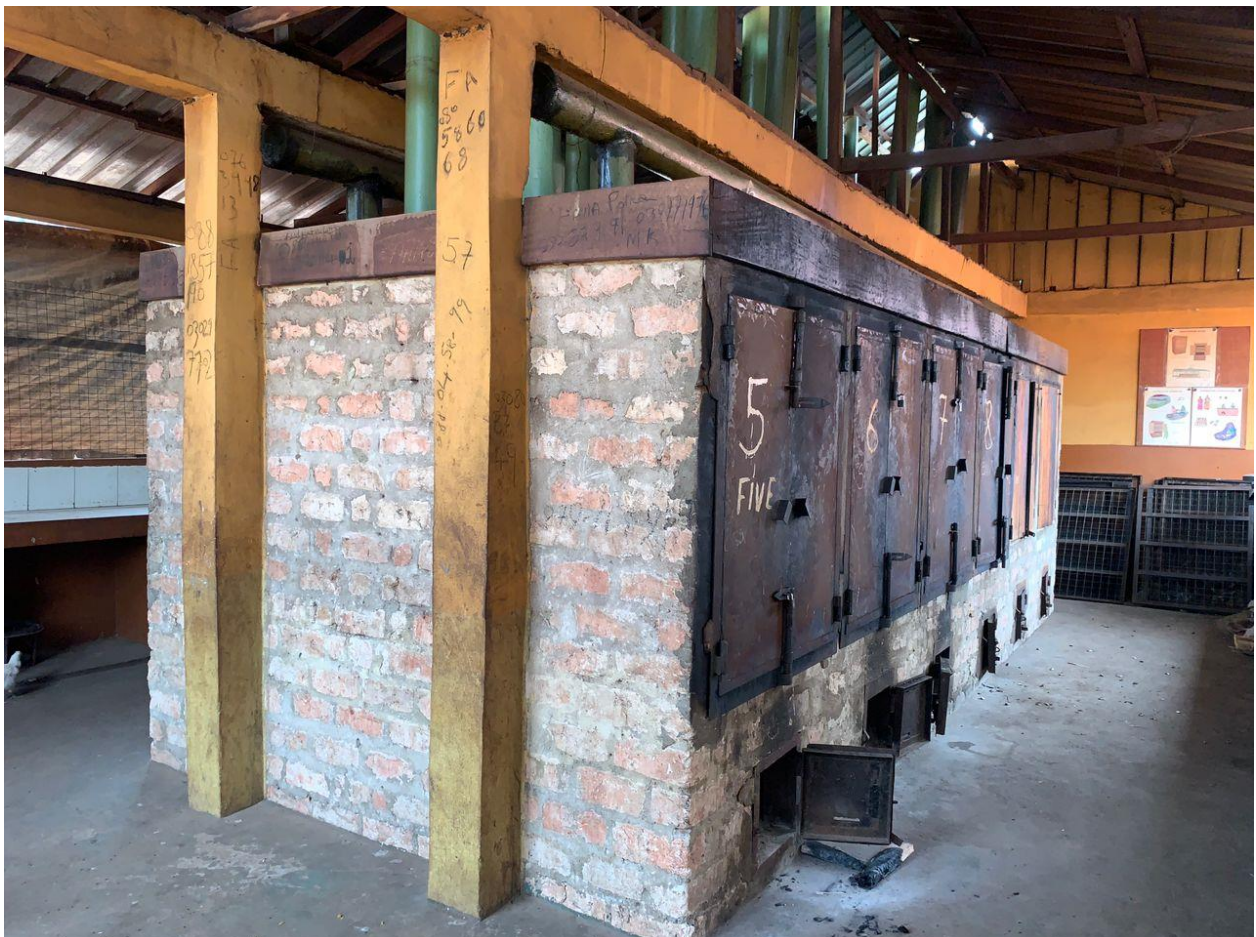
Figure 8: The improved kiln (Matis) smoke oven at Tombo
