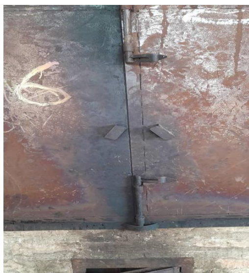
Figure 11: Closed oven during smoking (a); Fire chamber door with the air valve and lock (b).
