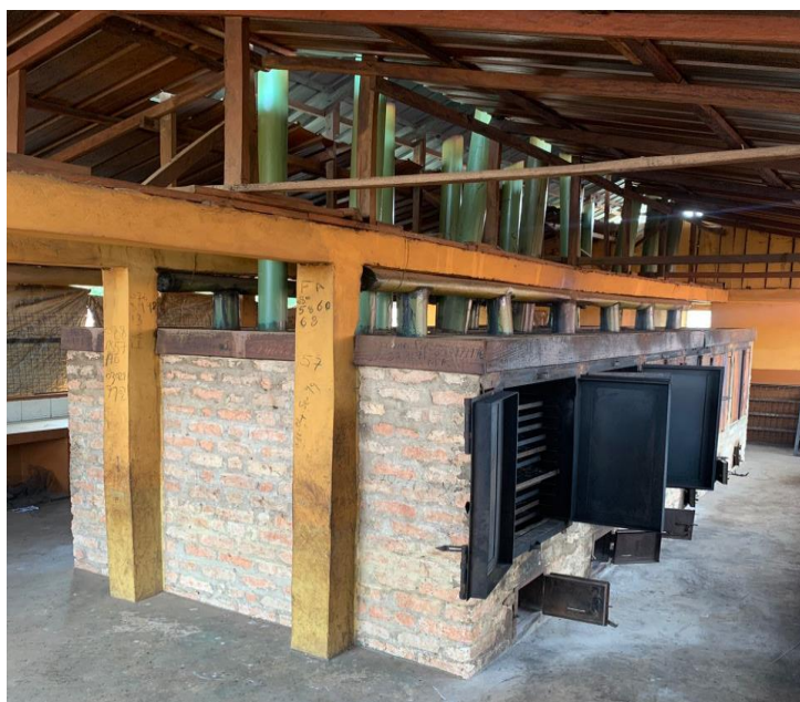
Figure 29: Matis oven with chimney GRÓ Fisheries Training Programme
