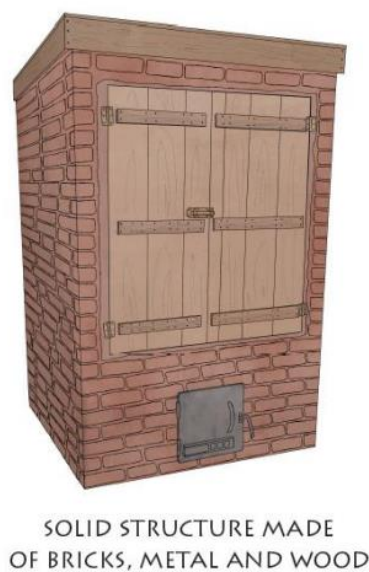
Figure 13: Solid structure made from bricks, metal, and wood (Gissurarson, 2019).
