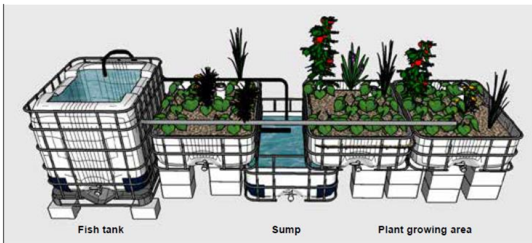
Figure 2: Media bed aquaponics unit, adopted from (Somerville, Cohen, Pantanella, Stankus, & Lovateli, 2014)
