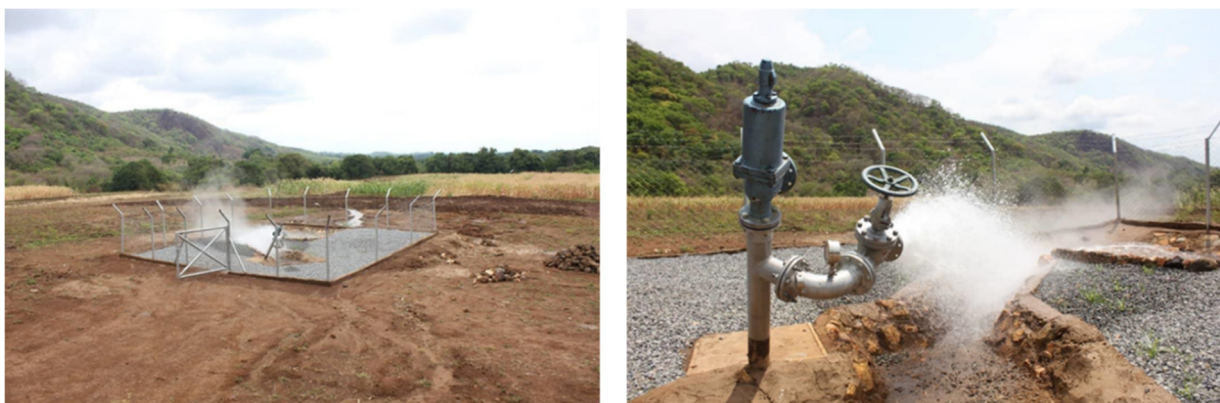
FIGURE 3: Photos showing a successful discharging shallow well drilled at Kiejo-Mbaka geothermal field
