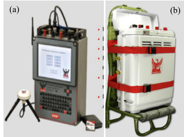
FIGURE 7: The V8 receiver (a) and T4 phoenix transmitter (b)
