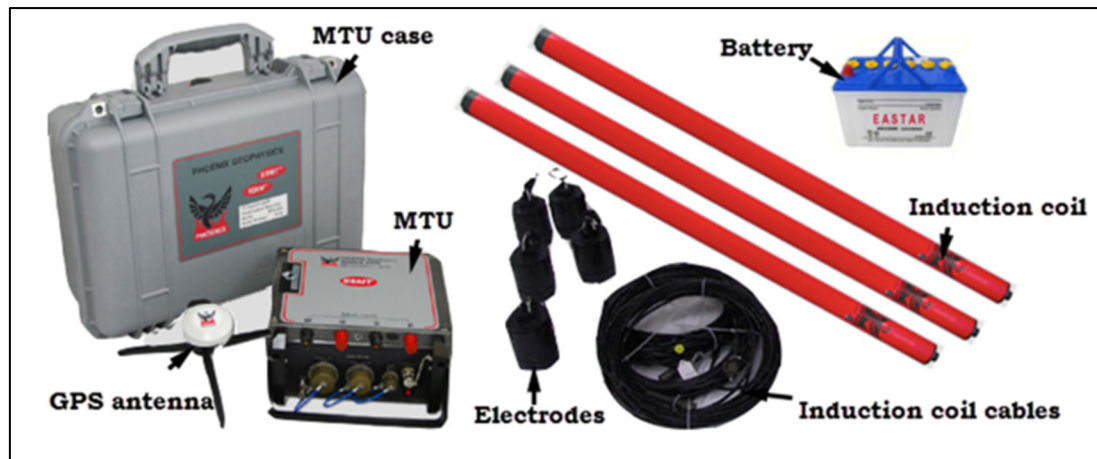
FIGURE 9: Instrumentation for a typical MTU-5A Station (modified from Phoenix, 2018)
