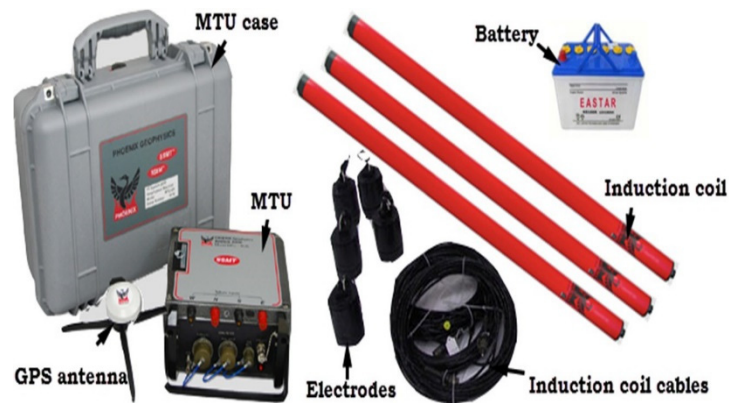
FIGURE 8: Phoenix geophysics equipment V5 2000 MT system (Phoenix, 2018)
