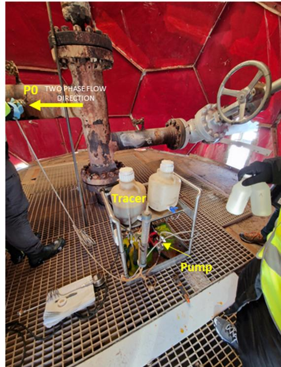
**Figure 3.5 Pumping tracer into well BJ-12**
