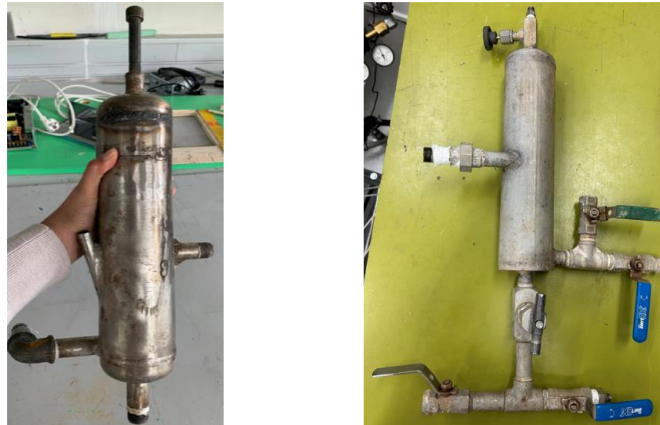
Figure 15: Experiment steam separators primary (left) and secondary (right)
