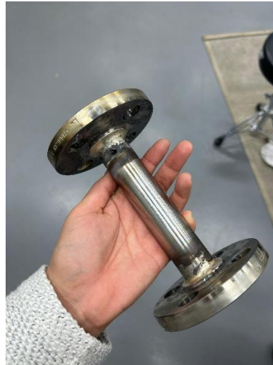
Fig B6 Primary flow section welded to flanges
