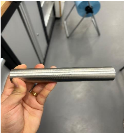
Fig B1 Machine and cut stainless-steel shaft
